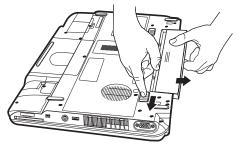
(Sample Illustration) Removing the battery
